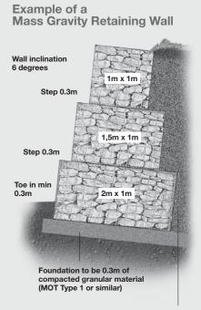
To rear of structure compacted granular fill in layers not exceeding 300mm
